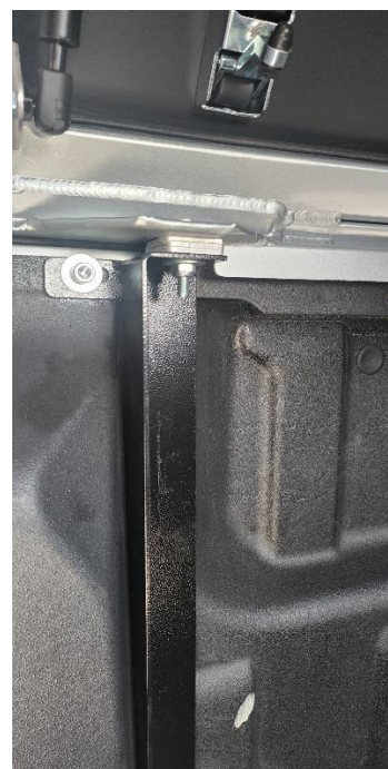
Pic 16 – Rear mounting bracket in position and tightened.
