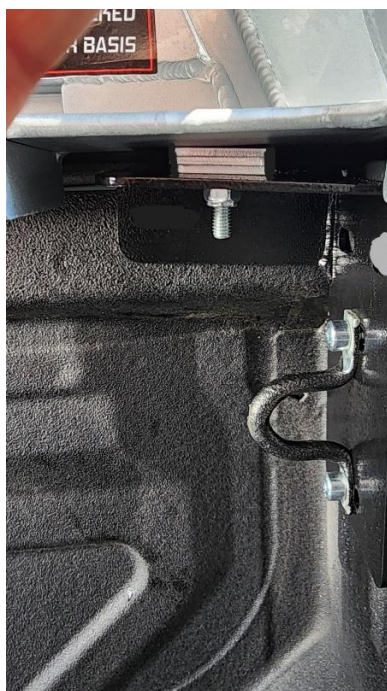
Pic 15 – Front mounting bracket In position and tightened
